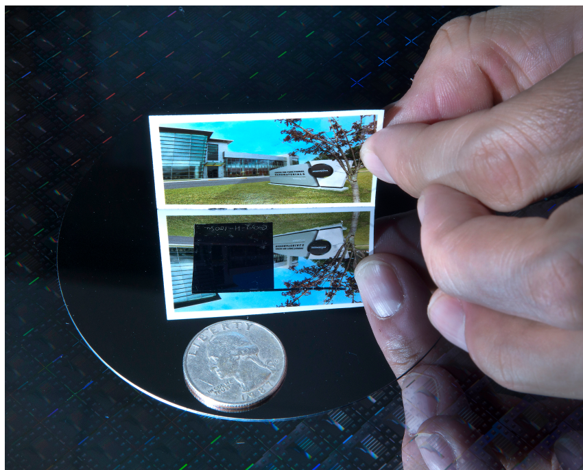
Figure 5. The reflective property of a Nano textured square of silicon influenced by moth eyes compared to a normal silicon wafer.
