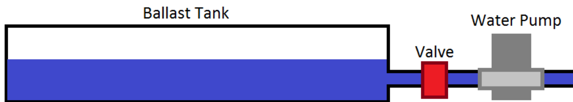
Figure 11: Simple Design of the Ballast System
