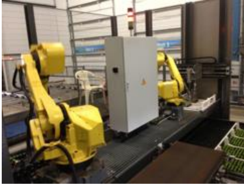
Figure 6: Robotic arms used to transfer the germinated seeds to the hydroponic rafts.
