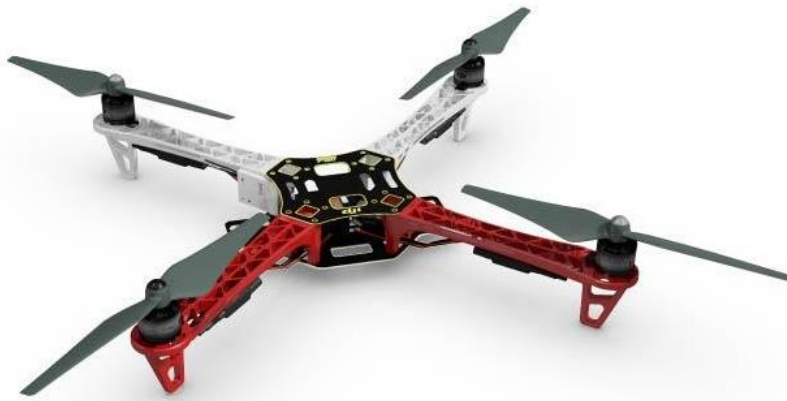
Figure 1: Hovercam Frame Kit
