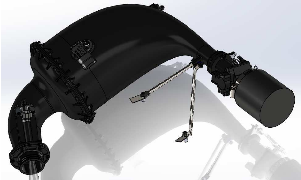
Figure 8: Final Assembly of Intake Manifold
