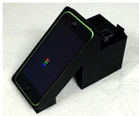
Figure 1. The SpecPhone apparatus is pictured. The housing is 3D-printed, and additional components are added in to complete the apparatus (Grasse, Torcasio & Smith, 2016).
