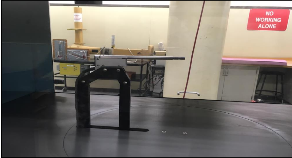
Figure 5: Wind tunnel probe ("sting") for mounting in wind tunnel
