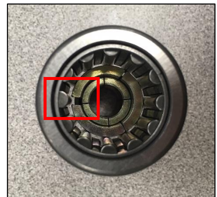
Figure 14: Rolling issue with mounting adapter
