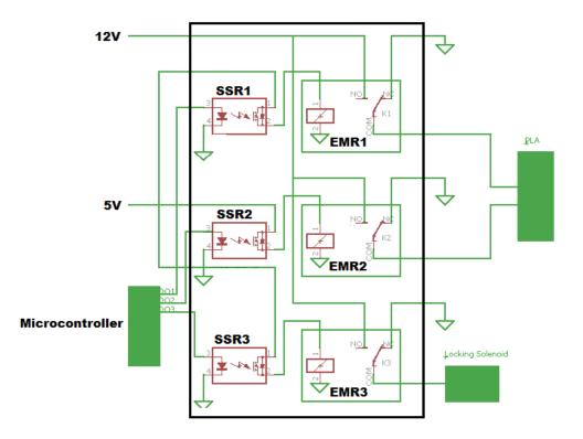
Figure 18: Relay Board Schematic
