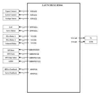
Figure 24: Microcontroller Pinout Diagram
