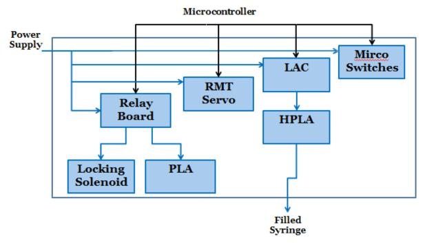
Figure 21: Level 2 Servos/Actuators/Sensors Design
