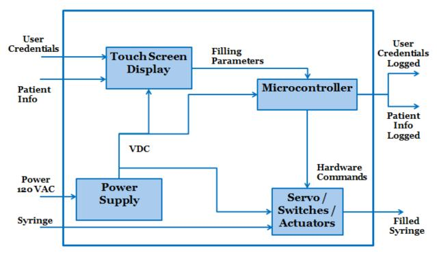
Figure 2: Level One System Diagram
