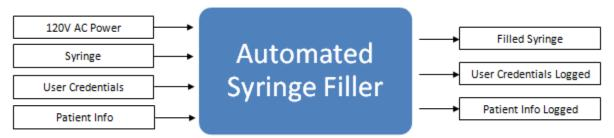
Figure 1: Level Zero System Diagram
