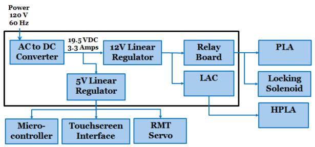
Figure 17: Level 2 Power Supply Diagram
