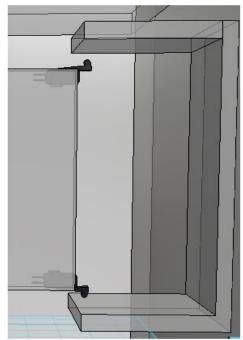
Figure 7: PLA Limit Switch Design
