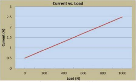
Figure 6: Current vs Load PLA
