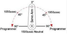
Figure 13: Servo Motor Rotation Diagram
