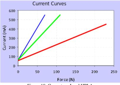
Figure 10: Current vs. Load HPLA
