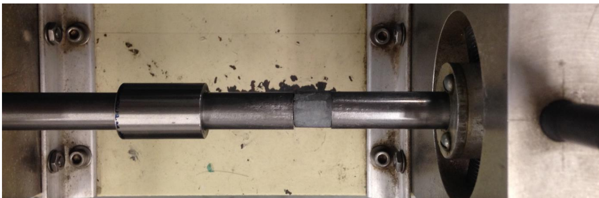
Figure 25: Sample placed between transmitter bar and incident bar
