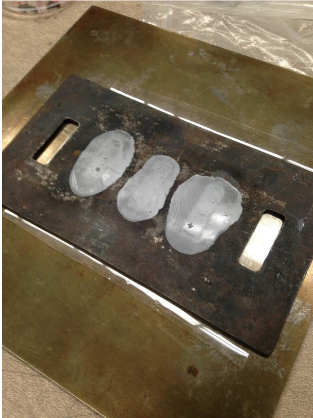
Figure 18: Cured epoxy in molds
