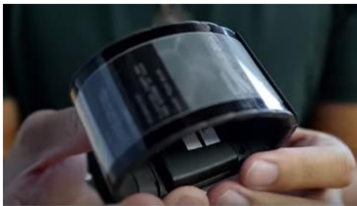
Fig. 1. A display from Polyera in its pre-alpha stage that wraps around a segmented bracelet
