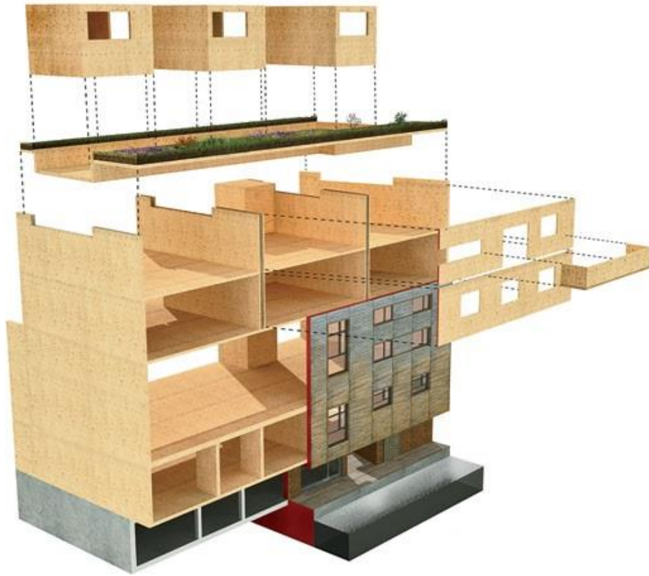
Figure 12: London's 52 Whitmore Road, designed by Waugh Thistleton with KHL UK, is a six-story CLT building [10].
