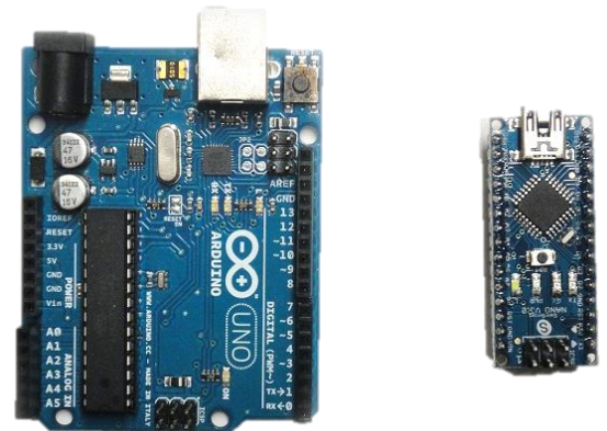
Figure 6: Visual comparison of UNO vs. Nano
