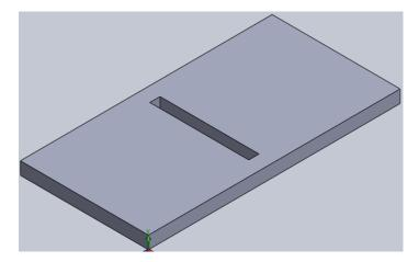
Figure 3: The slit that was 3D printed and inserted into the spectrophotometer. The slits measurements are 38.1 x 15.24 x 1.524 mm and a slit of 1.27 mm.
