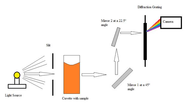
Figure 2: One side of the spectrophotometer developed. It is similar to the basic spectrophotometer except for the 45° angled which allows for the light to bounce in a straight line at mirror 2. The second mirror is at a 22.5° angle to allow for the light to strike the diffraction grating to allow for a measurement of the full visible spectrum. Note that this is the set up on both arms of the spectrometer.
