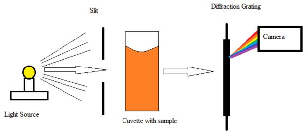
Figure 1: Light is produced form the light source and travels through the slit to allow only a controlled amount of light to pass through the sample. The light then passes through the diffraction grating causing dispersion of the light and travels into the camera allowing for analysis of the sample. The camera in this case was that of an Iphone® 5.
