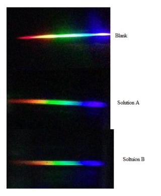
Figure 4: Pictures taken of the blank as well as solution A and B with the Iphone 5<sup>®</sup>. These were the pictures then used to analyze and obtain the graphs in figure 5. Note that the blank is more intense than sample A or B because of having no particles within the solution to absorb light.
