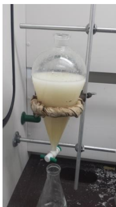
Figure 7: Example of the emulsion that forms during DI water/brine washes that can take hours or days to separate.
