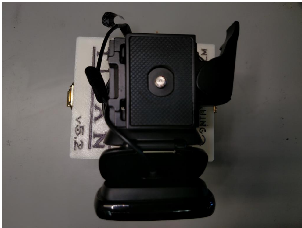
Figure 51 - Tripod-style camera mount on the top of the TITAN system's servo components
