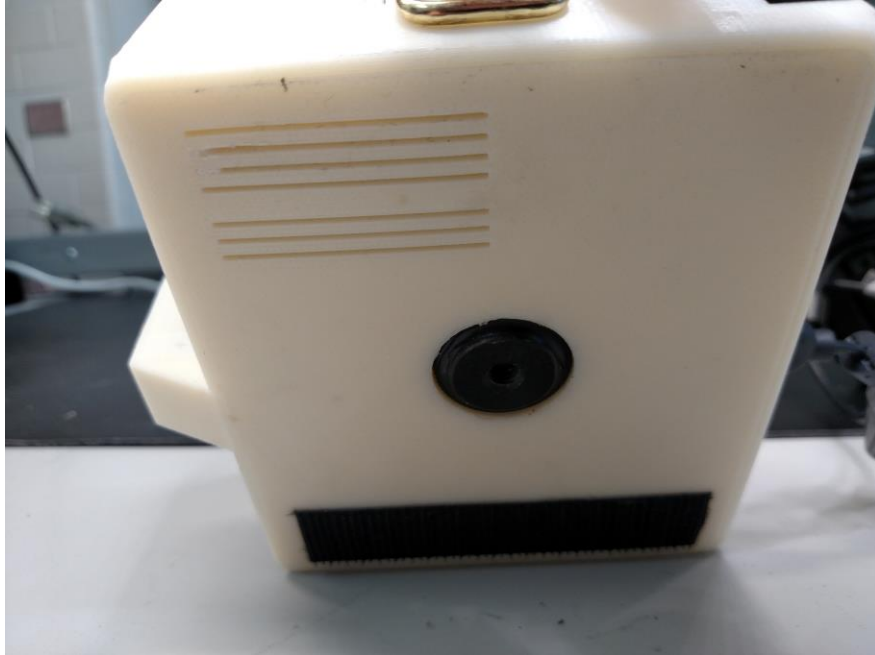
Figure 54 - The underside of the TITAN module's housing. Notice the air vents (top left), screw mount hardware (middle), and Velcro strip (bottom) which is used to attach a USB hub to the unit
