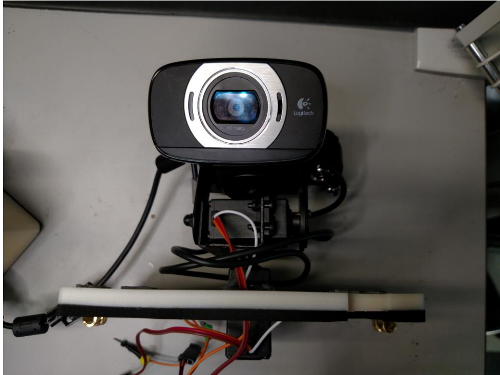
Figure 52 - TITAN's lid with servo and webcam mounted
