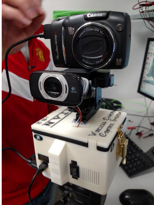
Figure 60 - Full prototype mock-up of TITAN system set up with tripod and external digital camera
