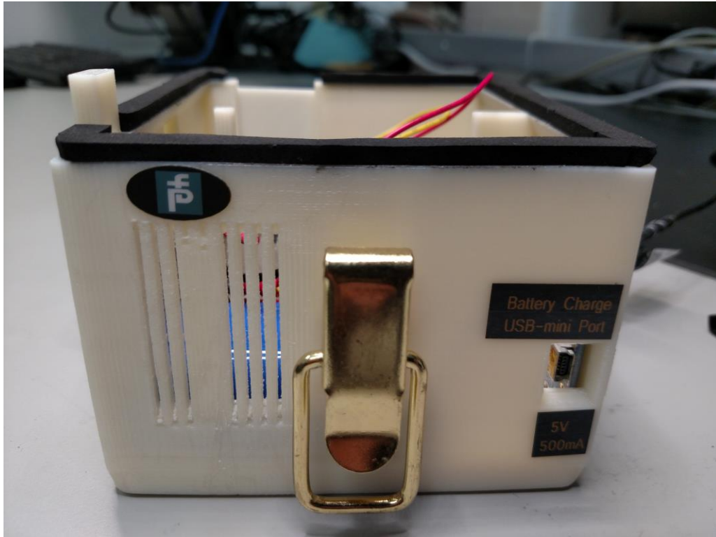
Figure 56 - The battery charger port side of the TITAN module
