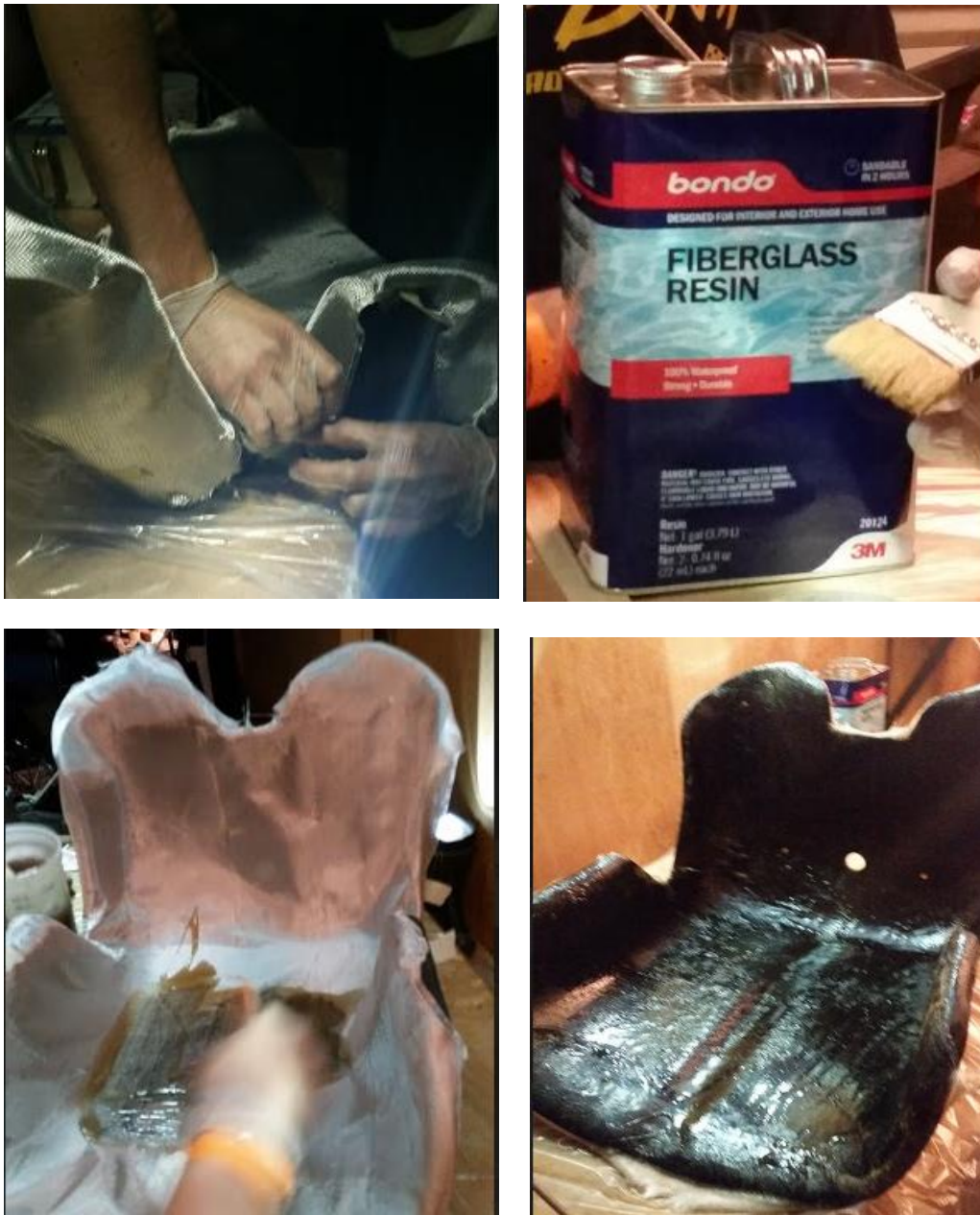
Figure 15: Fiberglass Cloth laid Over the Seat, Fiberglass Resin, Lay-up of the fiberglass, and final product
