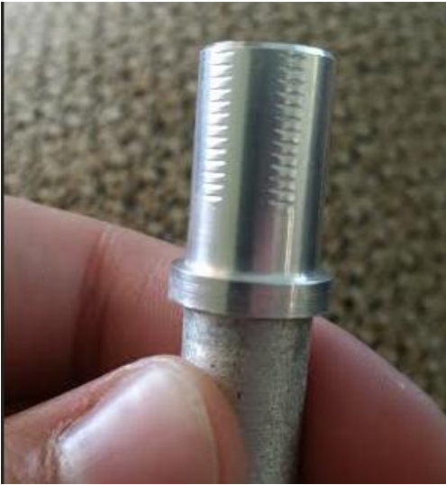
Figure 35:Procedures for Instron Testing- Grip Marks on Insert from Machine and Final Test Piece
