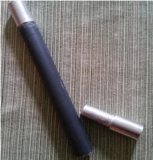
Figure 35:Procedures for Instron Testing- Grip Marks on Insert from Machine and Final Test Piece
