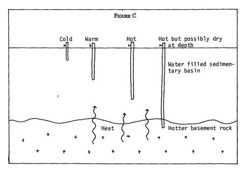
With Figure C we can have all three producing wells simply provide meteoric water at varying temperatures. Since the sediment filled basin may not be vertically homogenous with regard to "groundwater" quality, there may be considerable difference in the chemistry of the three wells in sediments. If the heat source is losing fluids, the picture becomes even more complex.
