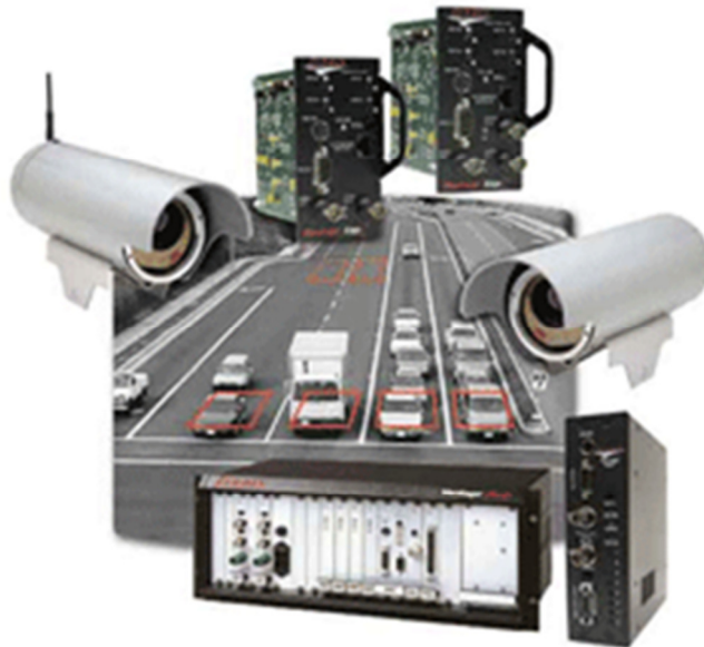
Figure 4: Video Image Processors (Muench, 2006)
