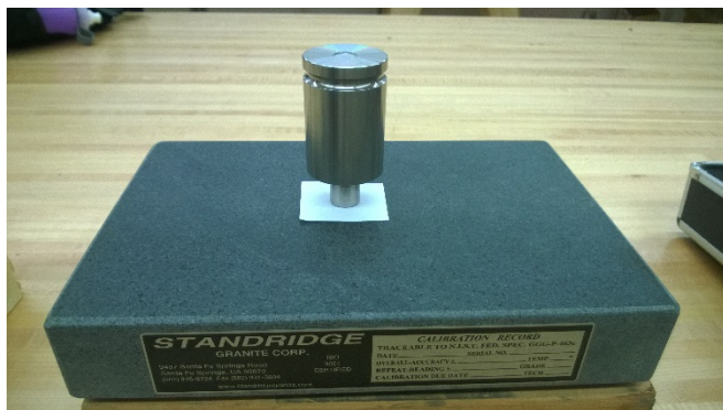
Figure 3: The set up that was used for creating the 8 to 28psi scale. A 0.75 inch diameter weight was used for the area our force was applied over. A flat was used for a level testing surface.
