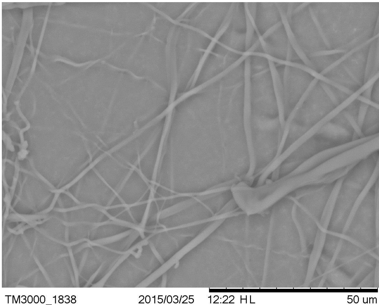
Figure 4: SIS nanofibers produced using 15wt% solution in 75:25 THF:DMF at 30kV and 25mL/h.
