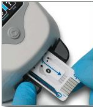
Figure 1: Image of the Coulter Counter Moxi Z miniaturized cell counting system. This commercially available system demonstrates the potential in miniaturized devices that can be directly translated to the team's microfluidic system.
