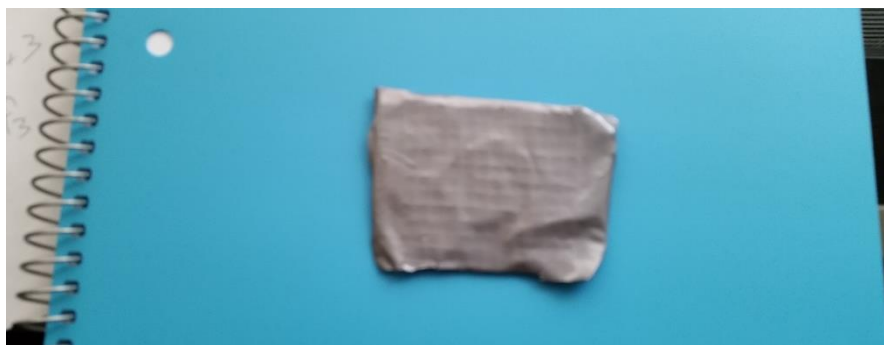
Figure 17: Five quarters wrapped in duct tape serving as a weight
