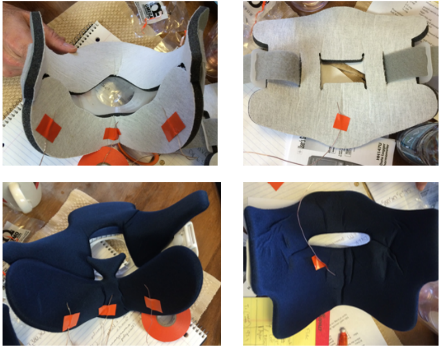
Figure E2. Quad-Thermocouple placement in Aspen and Miami J collars
