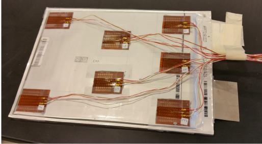
Figure 4: Sensor placement on battery
