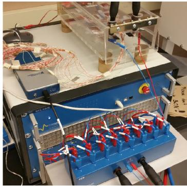
Figure 3: BCS-815 battery cycler with CC8 current collector
