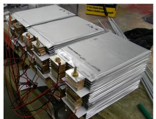
Figure 2: A typical lithium-ion battery pack for hybrid electric vehicles
