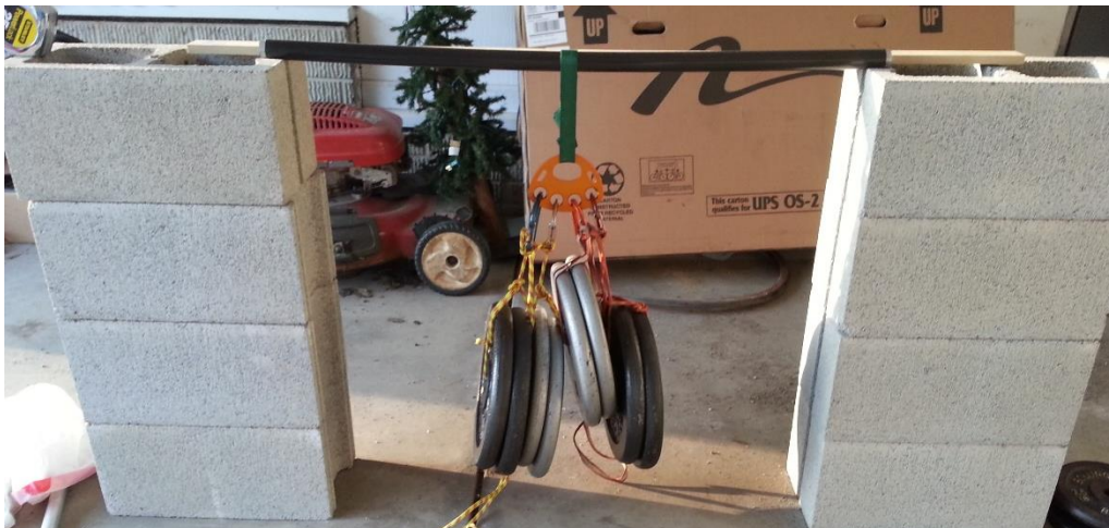
Figure 7: deflection seen by the Carbon fiber wrapped aluminum member under a 200lb load
