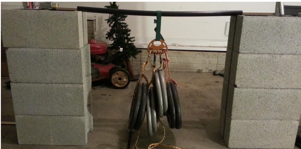
Figure 8: deflection seen by just the Carbon fiber tube under a 200lb load
