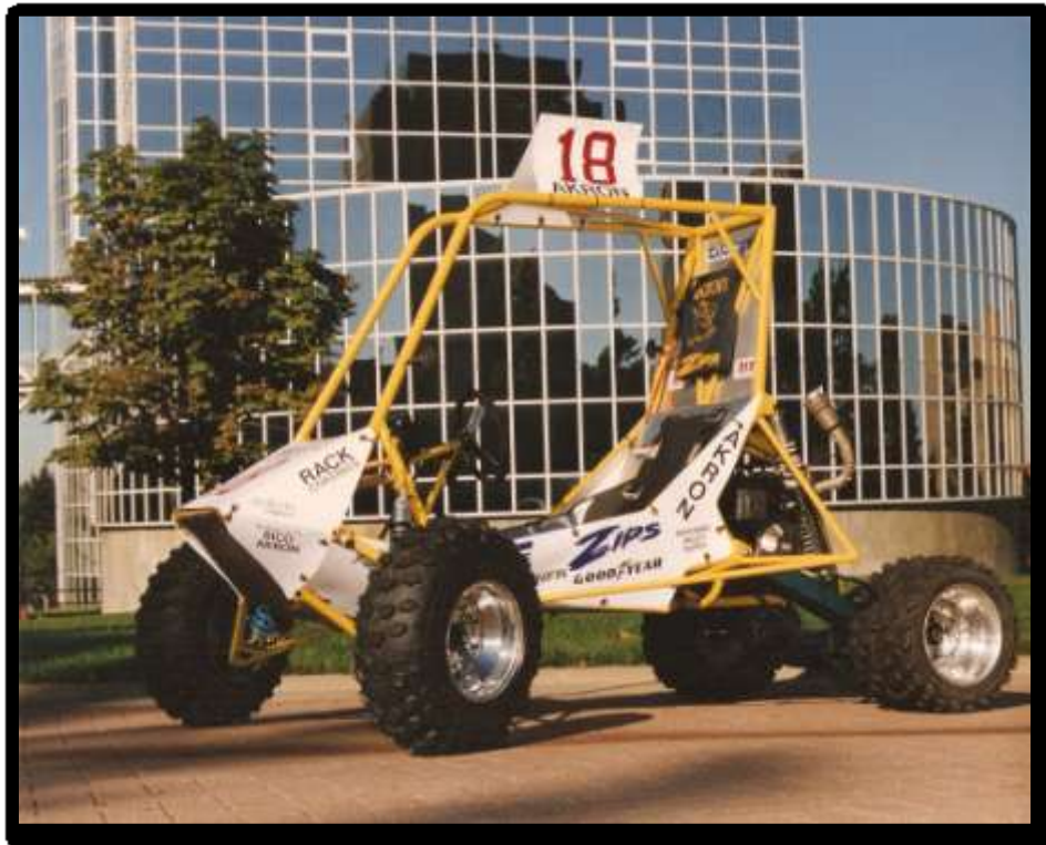
Figure 1: Picture of 1996 Zips Baja Car with Solid Rear Axle Swing Arm Suspension/Drivetrain
