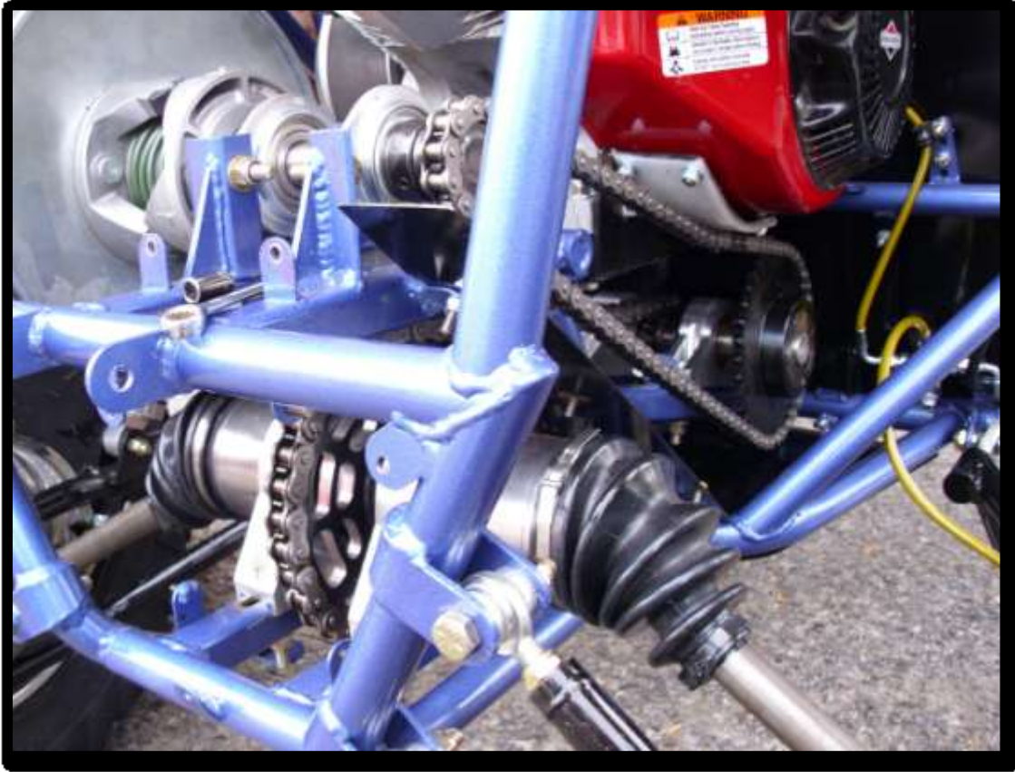
Figure 2: ZB14 Chain Drive Transmission w/ Comet 780 Series CVT and Polaris RZR Axles
