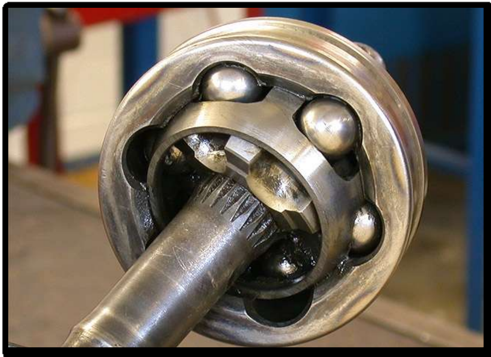
Figure 9: Outboard End of the CV Axle, showing the axle shaft (bottom left), bearing balls, inner cage, and outer housing
