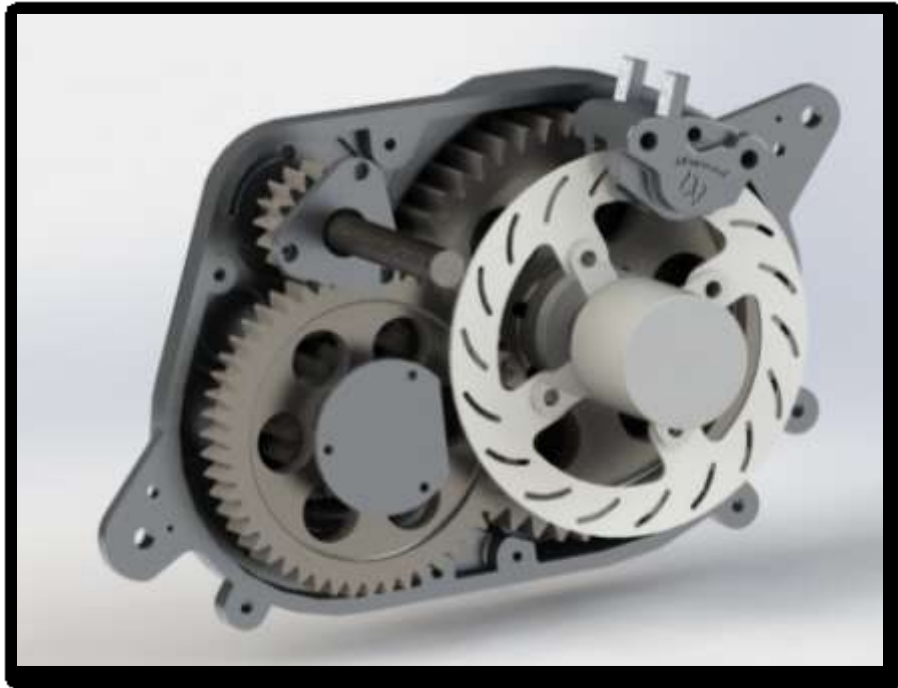
Figure 13: Rendering of Completed Gearbox Design in Solidworks (Half of the Gearbox Removed for clarity)
