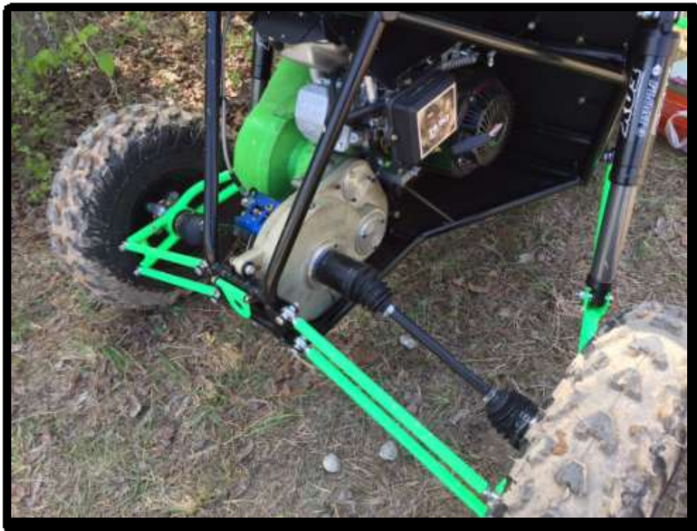
Figure 14: Completed Drivetrain on the Car at Auburn Alabama Competition
