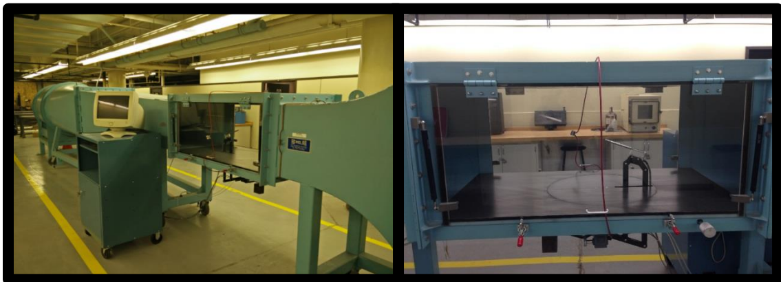
Figure 37: Working section of the Aerolab wind tunnel. Note the "sting" located in the center of the box
