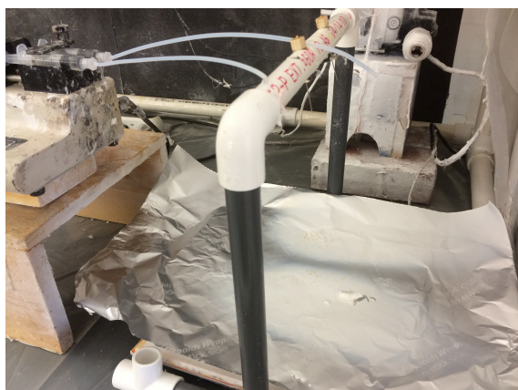
Figure 10. Sample of Nylon-6 from 10/17/2014 that inspired the 90-degree direction angle change for the nozzles not to break.
