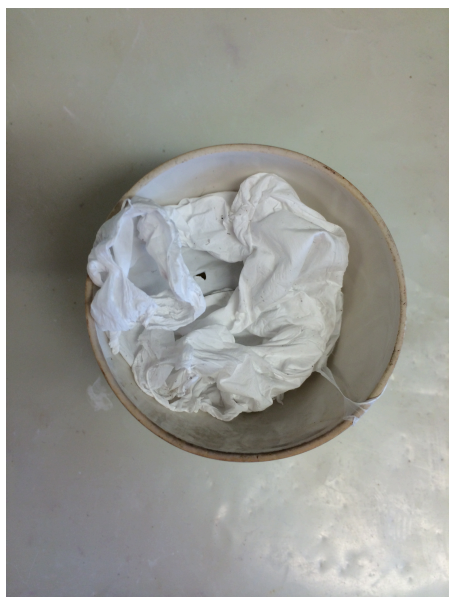
Figure 4. Fiber sample of PVDF-HFP to test various properties.
