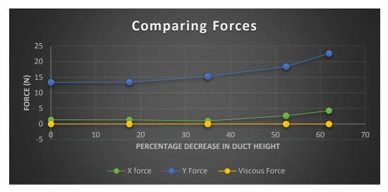
Figure 34: Force vs duct height
