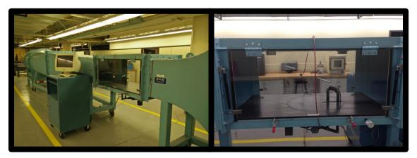
Figure 37: Working section of the Aerolab wind tunnel. Note the "sting" located in the center of the box
