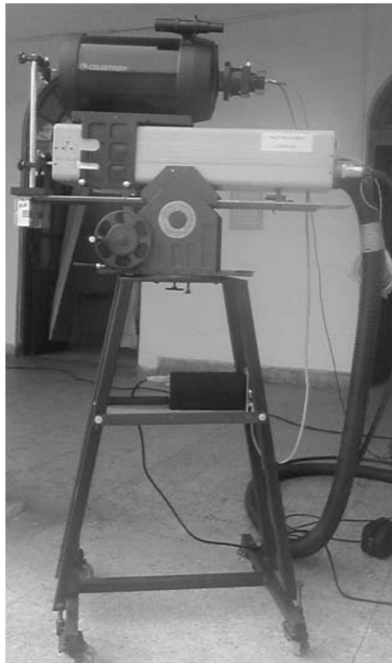
Fig 2: Photograph of indigenously developed backscattering lidar
