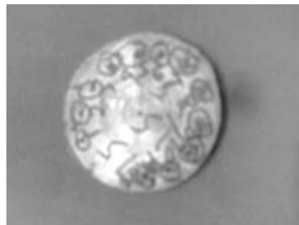
Fig-8, Casted work Piece ii sample cutted from casted work piece and drilled by fiber laser of 2 ton
