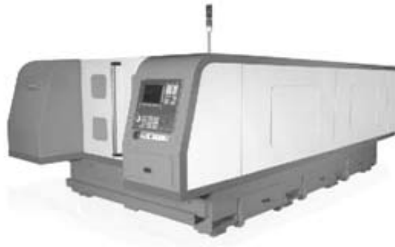
Fig 6, Fiber Laser Machine YLR 2000 used to cut the Al-AlO of volume 10%
