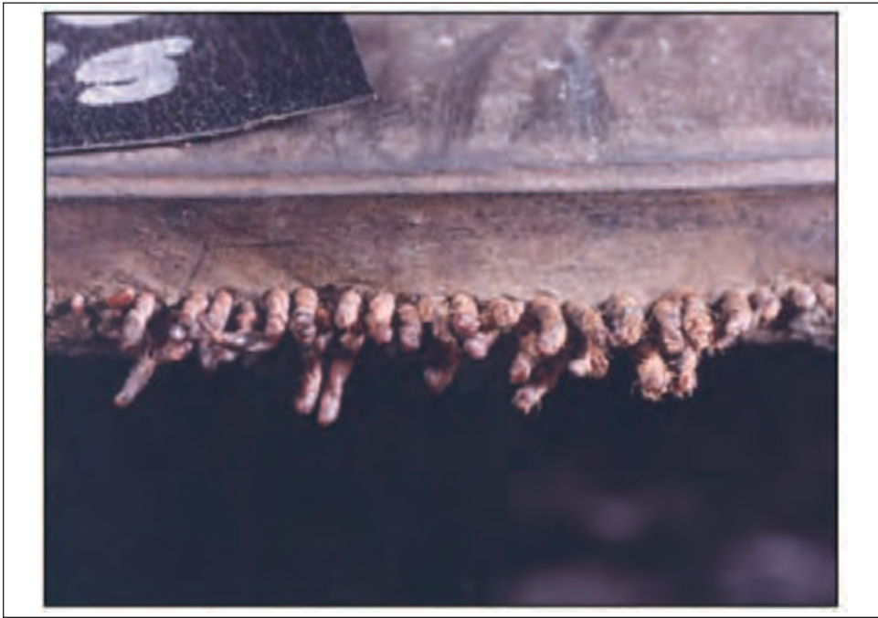
Figure 15.15: Broken, heat-fused polyester body cords, upper sidewall
