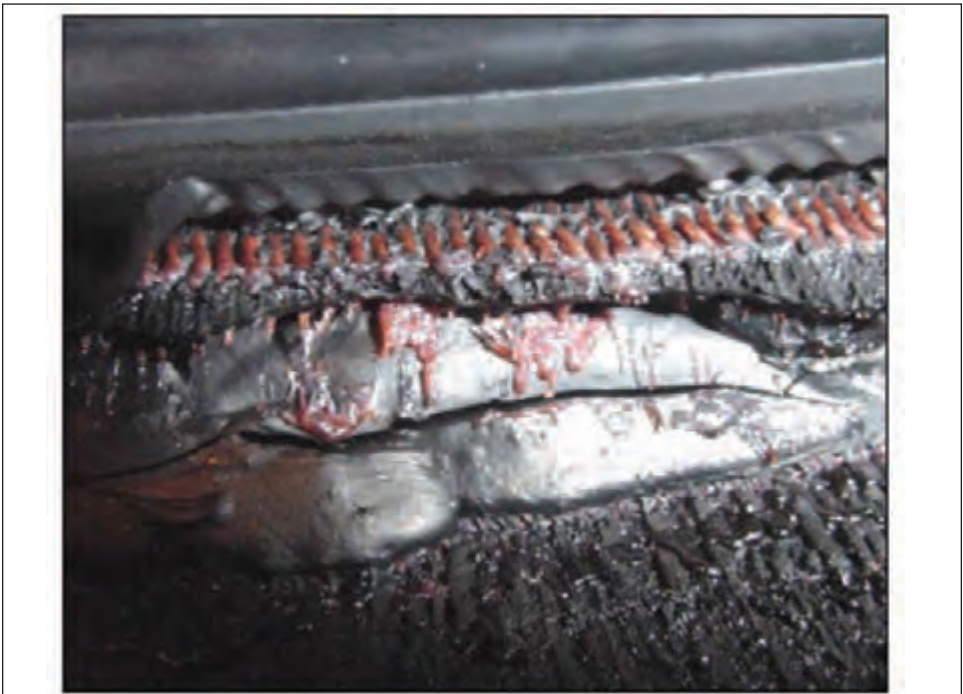
Figure 15.8: Melted polyester cord (lower sidewall)
