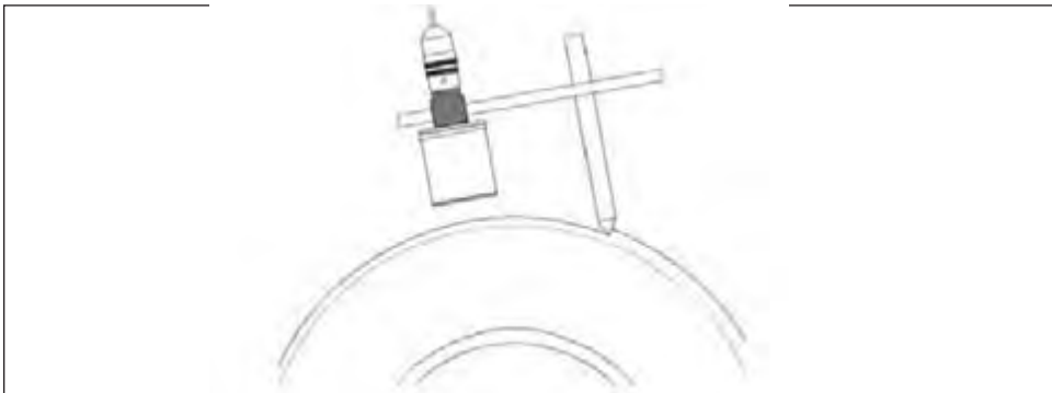
Figure 16.18: Eddy current measurement applied to a tire to evaluate retread thickness.
