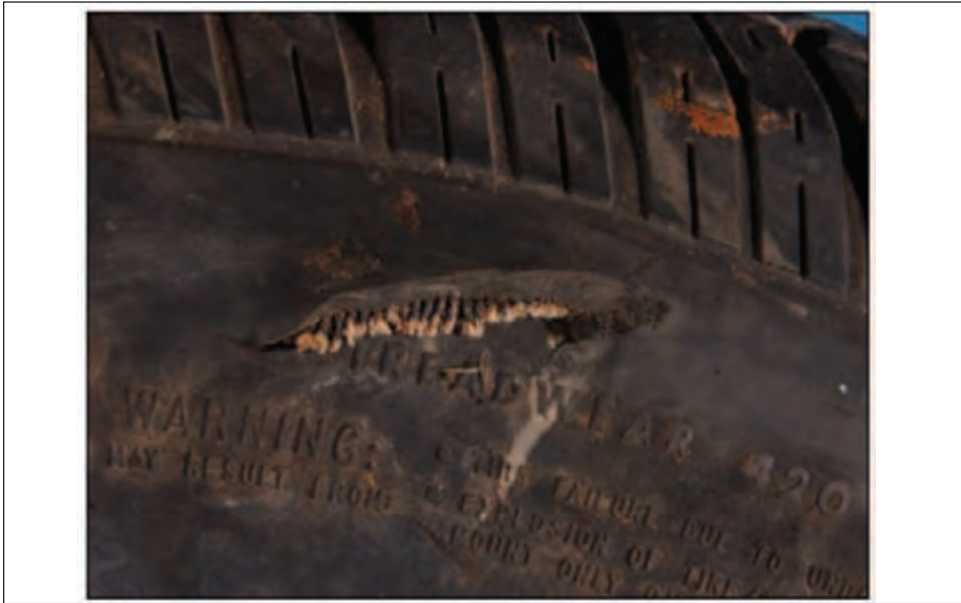
Figure 15.17: Upper sidewall break through to cavity
