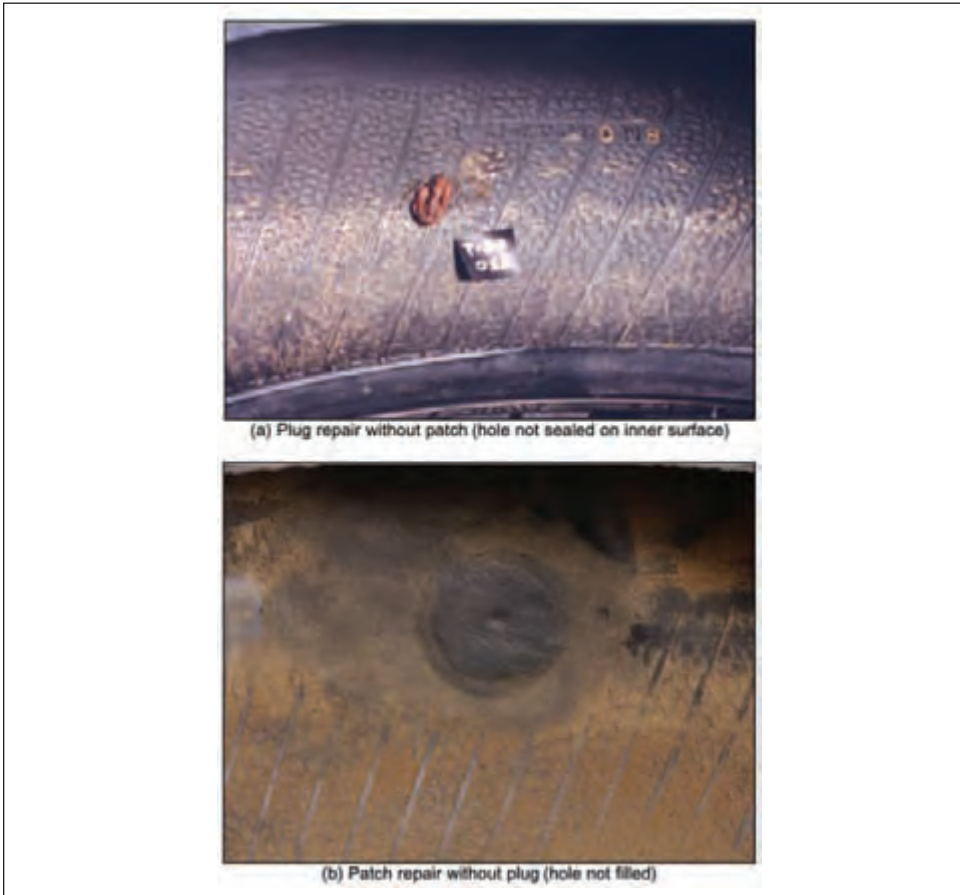
Figure 15.19: Examples of improper puncture repair
