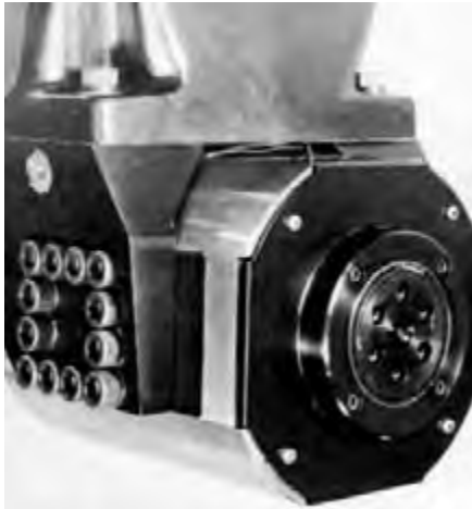
Figure 8.16: Unitary measuring head from a flat-trac II
