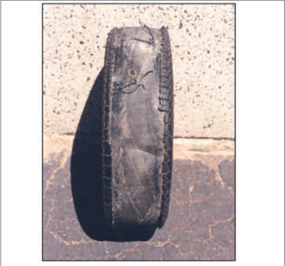
Figure 15.16: Exemplar tire after tread/belt detachment
