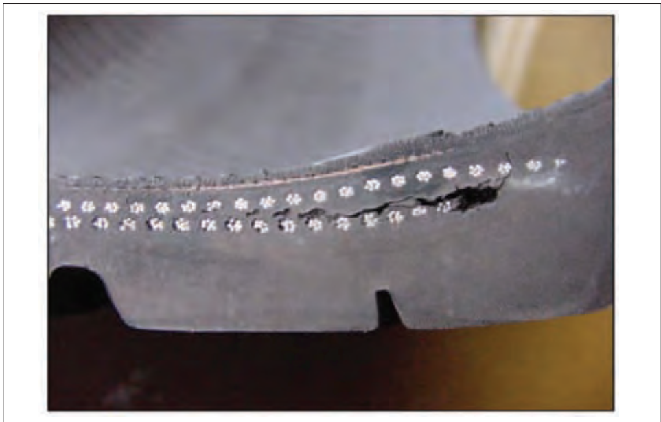
Figure 15.13: Cracking between steel belt edges
