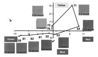
FIG. 2. Color change of the  $ZrN_x$  films with respect to the nitrogen content of the sputtering gas in the  $a^*$ ,  $b^*$  plane of the CIEL\* $a^*b$  color space (Ref. 18). The numbers next to data points indicate the relative brightness of the films.
