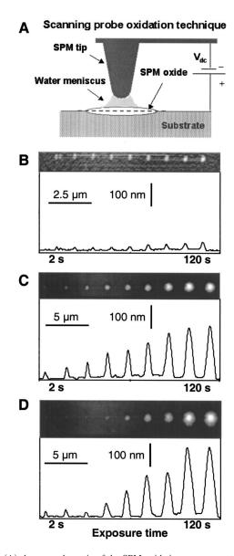
FIG. 6. (A) shows a schematic of the SPM oxidation arrangement used as a new characterization method in this work. Arrays of oxide features are produced as the voltage is applied for a fixed amount of time. The images of the oxide features generated on  $ZrN_x$  films with different nitrogen flow rates (0, 3.5, and 5 SCCM, respectively) are acquired in normal contact imaging mode after the oxidation and are shown in (B)–(D).
