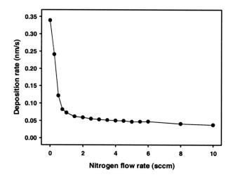
FIG. 1. Deposition rate of  $ZrN_x$  films deposited using rf sputtering at an argon flow rate of 2 SCCM, a power of 120 W, and a pressure increasing from 0.3 Pa at the lowest nitrogen flow rate to 0.6 Pa at the highest nitrogen flow rate.
