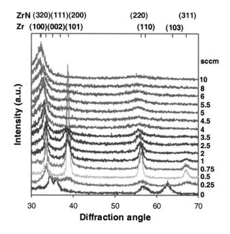
FIG. 3. Grazing angle XRD analysis of  $ZrN_x$  films deposited using rf sputtering. Spectra for films deposited with different nitrogen flow rates in the feed (SCCM) are shown. The gold stoichiometric film deposited at 0.5 SCCM nitrogen exhibits dominant ZrN(200) and (111) peaks in the presence of weaker (220) and (311) peaks.
