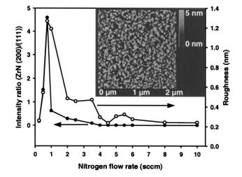
FIG. 4. Plot shows the effect of nitrogen flow rate on the ratio of the ZrN(200) and (111) peak intensities  $(I_{200}/I_{111})$  and the topography of the films (inset). The change in the root mean square surface roughness closely follows that of the  $I_{200}/I_{111}$  ratio.
