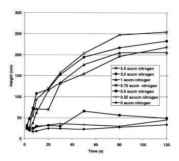
FIG. 7. Representative plots of oxide feature heights plotted as a function of time and nitrogen flow rate at an applied voltage of 30 V. Films deposited with 0.5 SCCM or lower nitrogen flow rate exhibit minimal oxidation, while there is significant oxide growth above this value.
