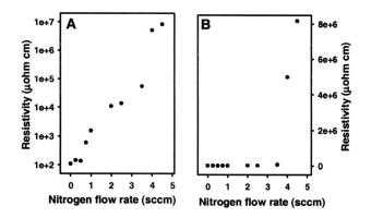
FIG. 5. Plot shows the variation in electrical resistivity as a function of nitrogen flow rate. (A) shows the variation plotted on a semilog plot, while (B) shows the linearly scaled graph.
