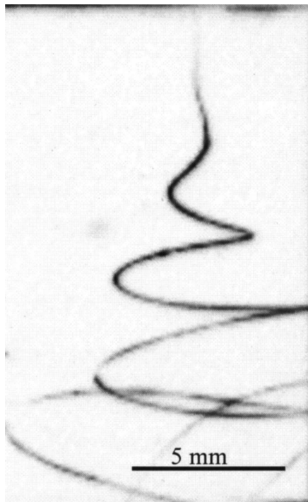
FIG. 3. Image of the electrically driven bending instability taken near the end of the straight part of the jet in experiment.
