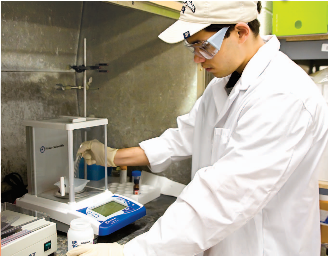
INBRE EXPERIMENTS: In a lab in Clarke Science Building, sophomore Nicole DeRoy loads electrophoresis gel; senior Luis Muñoz weighs agarose compound to produce a gel for electrophoresis analysis.
