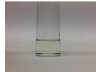
Kerosene cut (182-260°C)
