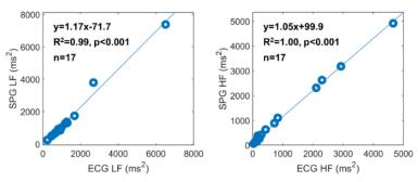
Figure 1 – SPG and ECG data collected from 17 subjects while standing. Waveforms were bandpass filtered to extract lowfrequency (LF) and high-frequency (HF) contributions to the waveforms. The data show a strong correlation.
