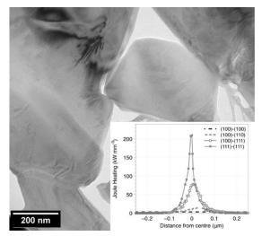
Figure 1 – TEM micrograph of FLASH sintered KNN, with amorphized GBs and penetration of sharp edge trough neighbor face. Overlapped calculated Joule heating for the four considered possible particle contacts.
