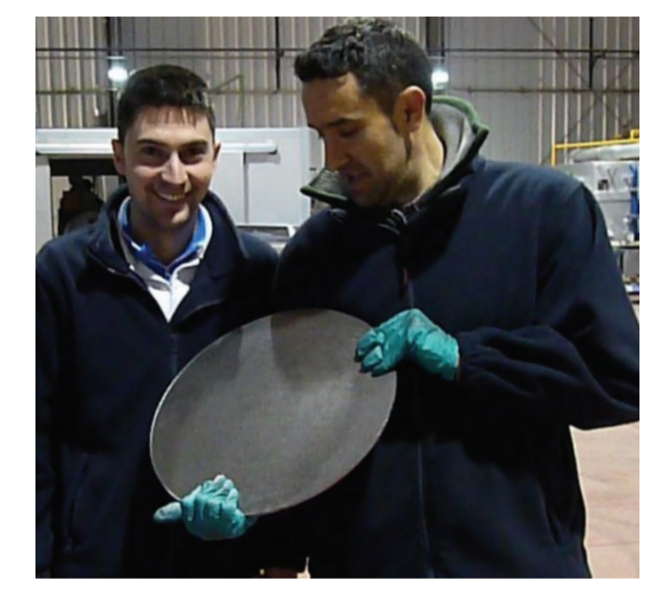
Early demonstration of the system performance: Pure Tungsten Carbide disc Ø 400 mm consolidated at 2100°C to full density
