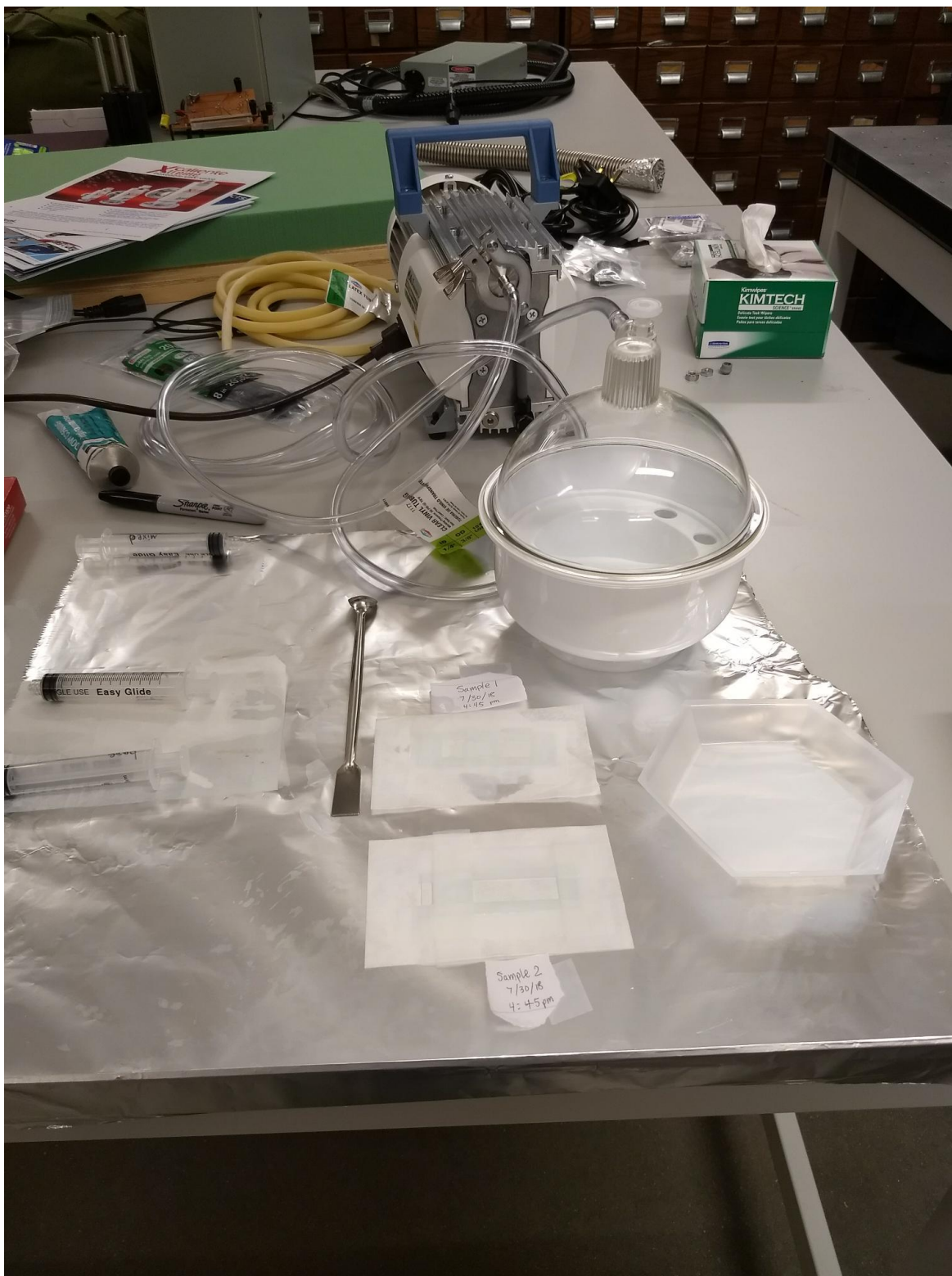
Figure 1 - PDMS Preparation: The set-up for preparing the PDMS samples. The vacuum pump is attached to the desiccator, and a weigh boat is in the front right.
