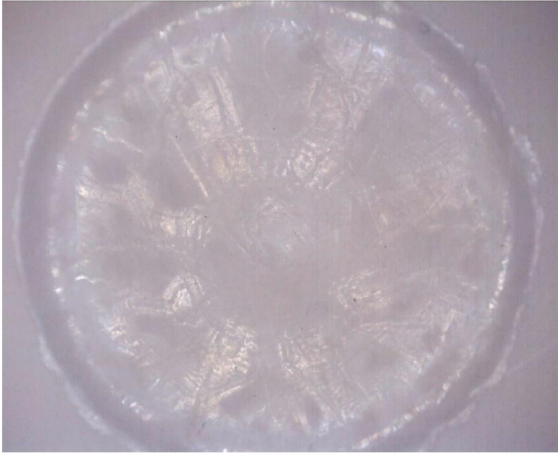
Figure 9 - Guanine Embedded in PDMS
