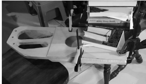
Figure 17: Gluing the Sound box together
