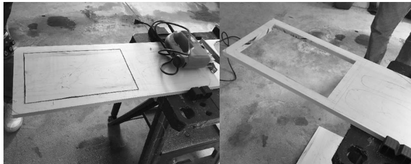
Figures 10: Cutting Out the Sound Box
