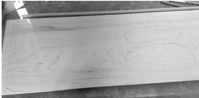
Figure 9: Body of Jouhikko Traced on Maple Wood
