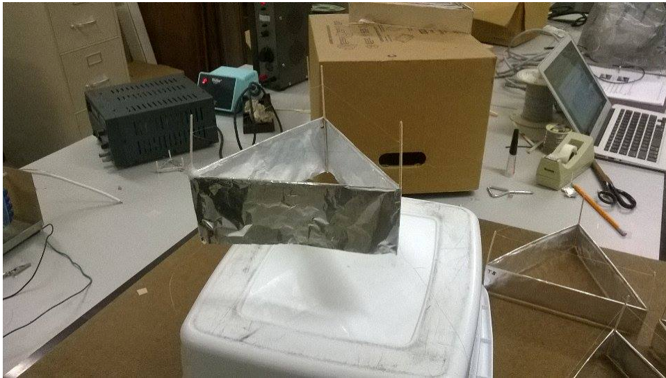
Figure VI - The lift was not as efficient. The longer width of the aluminum did not help with the lift.
