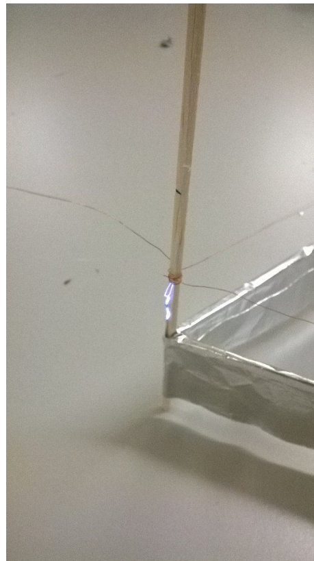
Figure II. Arcing on the Craft
