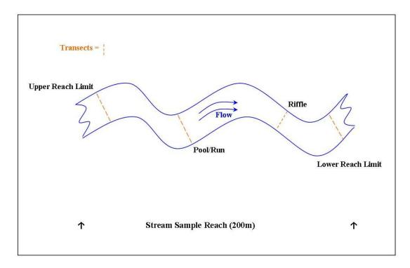
Figure 4 Idealized representation of typical stream sampling reach indicating upper and lower sampling reach limits, two flow regimes, and relative position of physicochemical measurement transects.
