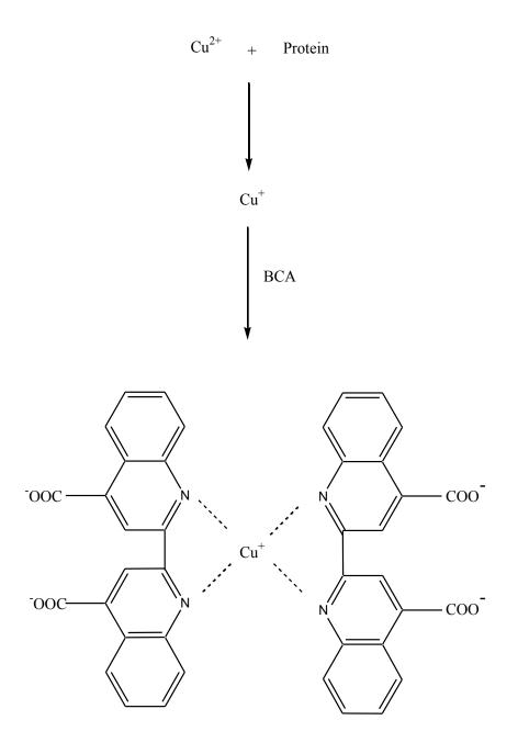
Figure 3.1 Reaction of BCA complex with Cu<sup>+</sup> (Smith, Krohn et al. 1985).
