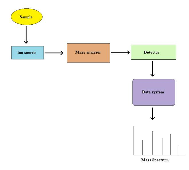
Figure 2.12 Block diagram of a mass spectrometer.
