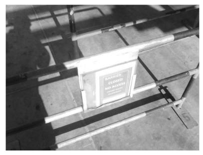
Figure 4. Typical Barrier for Lifting Operations. This is a typical barrier is used to close access to areas on the rig. Barriers restrict access due to overhead operations.
