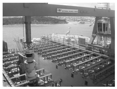
Figure 3. Rig's Riser Bay. Risers connect the rig to the ocean floor via the BOP and well head.
