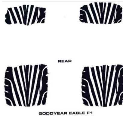
Figure 2.10: Vehicle at Acceleration Tire Patches
