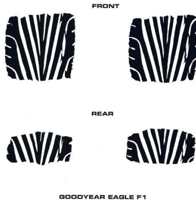
Figure 2.11: Vehicle at Deceleration Tire Patches
