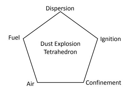
Figure 2: Dust Explosion Tetrahedron
