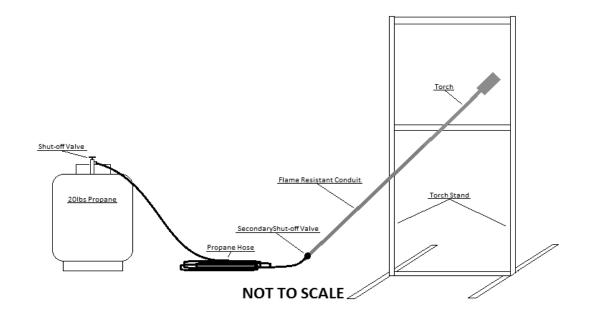
Figure 4: Propane Ignition Device
