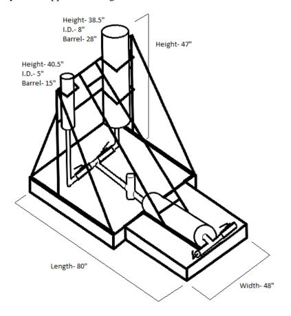
Figure 3: Dust Dispersion Apparatus Design
