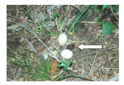
Figure 1. iButton placement in the ground at a Chuck-will's-widow nest. Arrow is pointing to the iButton located between the eggs.
