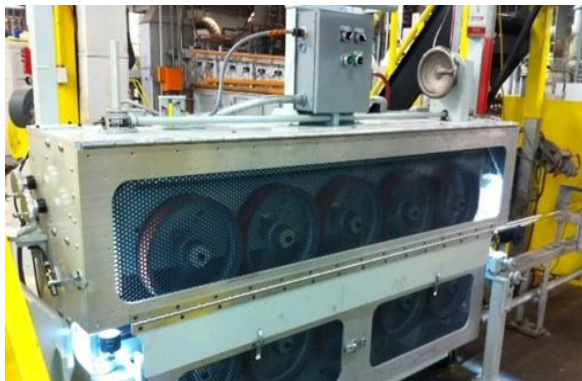
FIGURE 4: THE NEW & IMPROVED TRACTOR DESIGNED BY OSRAM ENGINEER MATT HUGHES (HUGHES, 2015)
