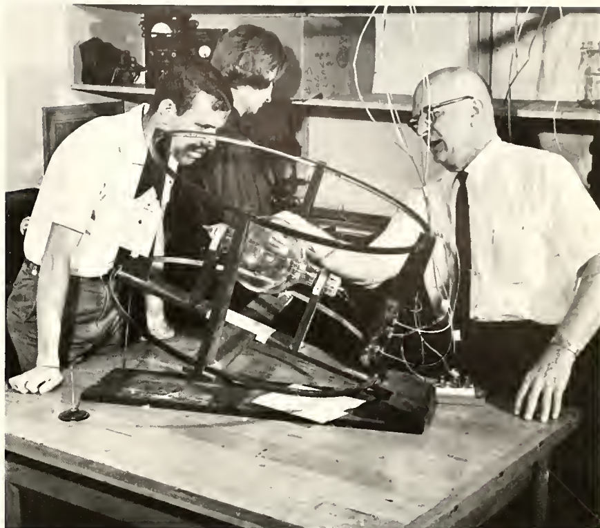
Dr. J. G. Black uses a simple laboratory model to demonstrate the principle of the vacuum tube.
