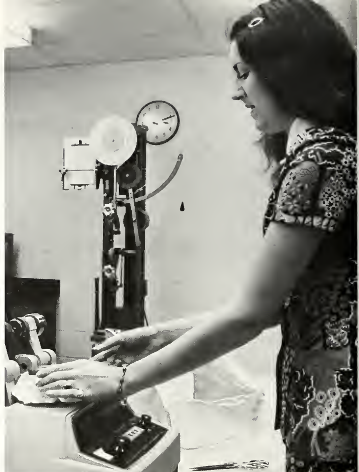
Pam Caldwell tests the abrasion resistance of cloth with the use of the Taber Abraser.
